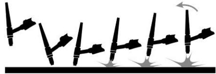
**START AND FINISHING OF WELDING PROCESS TIG (picture 3)**
